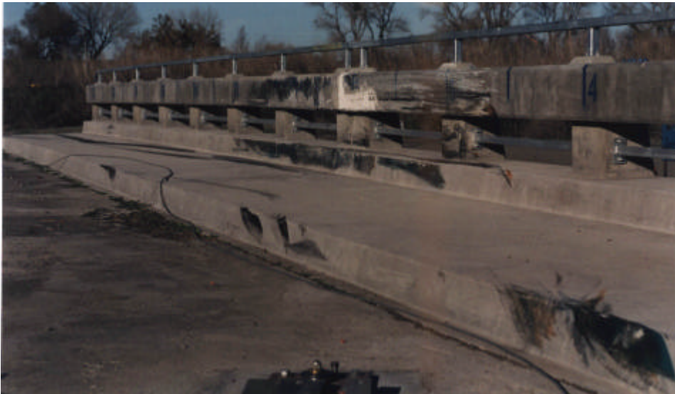
Figure 2-23 - Post Impact Bridge Rail Scuff Marks Test 541
